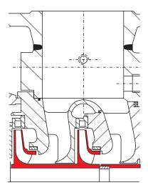
All across the delivery-data range (selection chart) additional outlays for ensuring adequate suction head are seen to be unnecessary. In many cases, a booster pump can be dispensed with merely by opting for a suction impeller or a double-flow in-take. Even for the latter, standard impellers are used.
