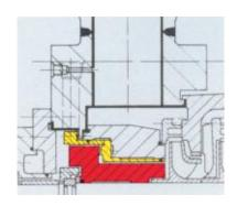
Hydraulic balancing devices compensate for axial thrust. Depending on the pump design and the user's individual requirements, balancing is attended to by a disk, piston or double piston.
