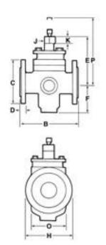
Valves have face-to-face dimensions conforming to BS 5158 PN 10/16, BS 2080 Class 150 Short, ANSI B16.10 & API 6D Class 150 Short. These valves are thus interchangeable with equivalent gate valves. Valves have Patterns conforming to BS 5353, BS 5158, API 6D & API 599 Short (with steel plug).
