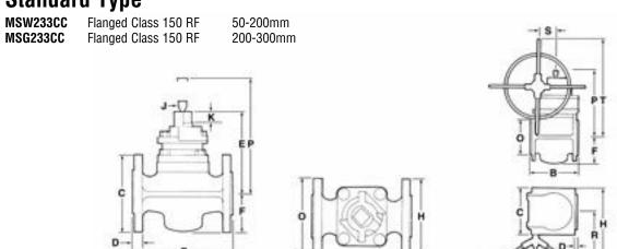
Flanged valves have face-to-face dimensions conforming to BS 5158 PN 10/16 & BS 2080 Class 150 Short, ANSI B16.10 & API 6D Class 150 Short. These valves are thus interchangeable with equivalent gate valves. Flanged valves have patterns conforming to BS 5353, BS 5158, ANSI B16.34, API 6D & API 599 Short (with steel plug).
