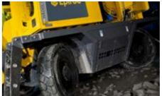
Wheel mounted with high tramming capacity, low diesel consumption, independent front and rear axle steering and four-wheel drive.
