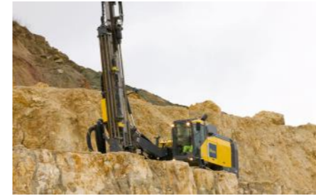
Built for high efficiency mining, the DTH hammer fitted to the FlexiROC D65 benefits from a precisely matched compressor.
