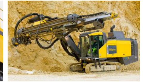
When equipped with the standard feed option, the FlexiROC D65 is capable of handling an even wider range of jobs with ease, including drilling de-watering holes.
