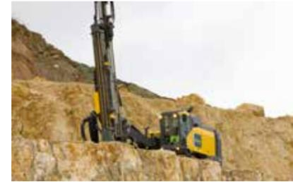
The FlexiROC D60 is built for high efficiency mining. Its DTH hammer benefits from a precisely matched compressor.
