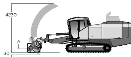
Toe-hole drilling (mm) (standard feed only)
