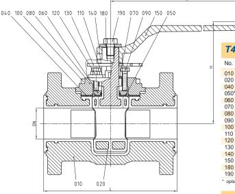
T4E3 DN<sup>1</sup>/<sub>2</sub>" to DN6" - material specification
