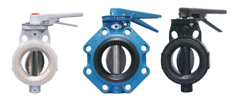
AUDCO Butterfly Valve is a Wafer type Valve with an integrally moulded elastomer body liner. Designed to outperform loose liners, AUDCO Butterfly Valve elastomer liner is moulded directly in the body bore and vulcanised in-situ, making it last the entire life of the valve. The result - a valve that requires no form of maintenance. A perfect FIT AND FORGET valve.
