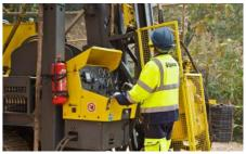
Ergonomic and user-friendly design, which displays the drilling parameters necessary to ensure productive drilling. Also included is a hold back function to prolong bit life.
