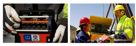
The Boyles C6C crawler rigs come with a radio remote control, which allows you to tram the rig from a distance providing a safer working environment.
