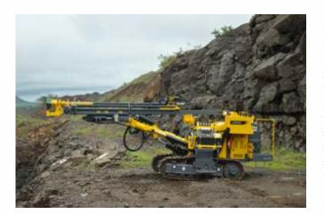
AirROC D40 SH is powered by the reliable onboard 50 HP Mahindra Diesel engine. The hydraulic system is well synchronized to meet the demand of this drill. It has a heavy duty feed mechanism which can generate tractive pull of 20kN along with powerful rotation unit which provides high rotation torque to tackle challenging rock formations.
