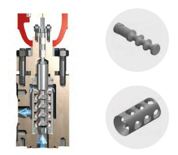
relatively large flow passages and shearing action provided by the multiple stage plug & cage designs, these valves are particularly well suited for applications involving fluids with entrained particles. This is of more relevance in older power plants when pipe scales can pass through the feed water.
