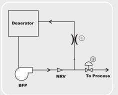
1- Fixed Pressure Reduction Device 2 - Feedwater Regulating Control Valve
