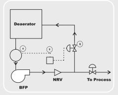
5 - For ON-OFF: Flow/Temp/Pressure Switch of On/Off Controller For Modulating: Flow/Temp/Pressure Modulating Controller 6 - BFP Min.RC Valve
